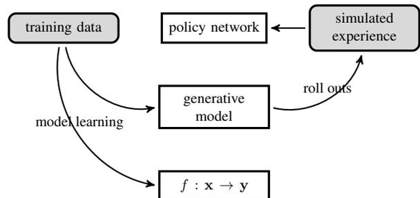
Figure 1. Diagram of the proposed RL framework for dynamic feature acquisition.
